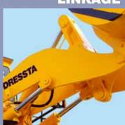
Z-Bar linkage transfers maximu force to the bucket to pry out had material.
