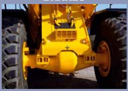
Internal wet disc brakes are forced cooled and enable the loader to be operated in any type of work cycle without overheating. Being sealed from outside contaminants protects the brakes and also extends brake life, especially in very abrasive or caustic environments, encountered in cement or chemical plants.
