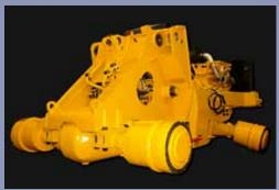
cylinder pivots increased lifting ability to the top without sacrificing digging ability. The rear frame features trunion rear axle mountings.
