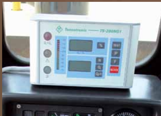
Optional electronic safe load indicator (ESLI) shows necessary load handling information.
