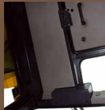
Cab roof window provides full view of all operations while the emergency stop provides operator's safety.
