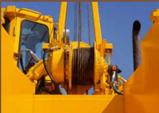
Two independently controlled hydraulic winches drive the boom and hook systems.
