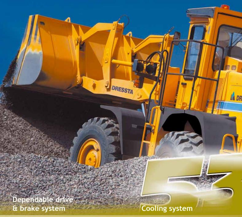
Planetary final drives, fully floating drive axles with conventional differentials provide most efficient mechanical transfer of torque and best fuel economy under good traction conditions. Operating independently, front and rear brake circuits ensure the safe loader operation through step less loader speed control.
