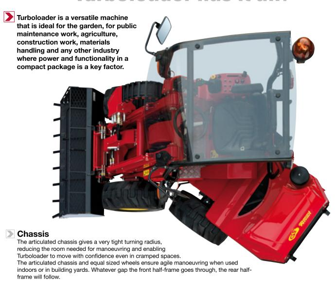
The rear wheels always follow the same path of the front ones, minimising compaction of the ground. Its articulated steering means Turboloader can work even on the most delicate surfaces without damage, making it ideal for landscaping and maintenance of green areas.
