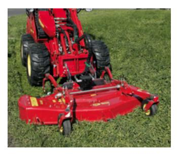
Side discharge + mulching mower deck Conversion kit included
